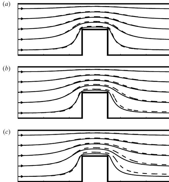
FIGURE 5. Streamline patterns at the mid-plane of a constricted channel ( $l, d = 0.5$ ) as obtained from the analysis (solid) and numerical simulation ( $\varepsilon = 0.05$ , dashed) for (a)  $Re = 0$ , (b)  $Re = 10$  and (c)  $Re = 20$ .
