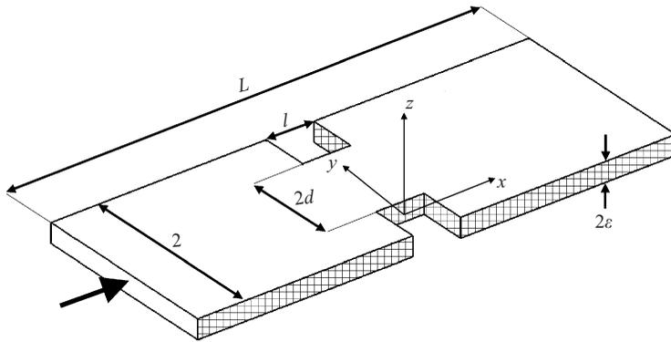
FIGURE 1. A schematic view of the constricted micro-channel defining the geometrical parameters  $l$ ,  $d$  and  $L$  and the coordinate axes. (All dimensions are scaled by  $D$ , half the channel width.)
