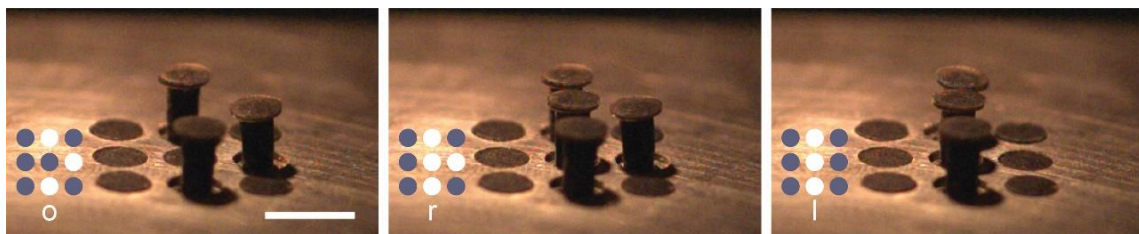
Fig. S11. Braille Tactile Display States. Programmed actuation sequences produce braille text. Image brightness and contrast increased to improve visibility. Scale bar: 5 mm.
